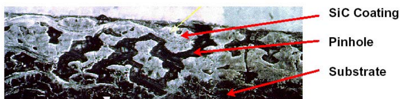
Photo Micrograph of Pinhole Through Coating
